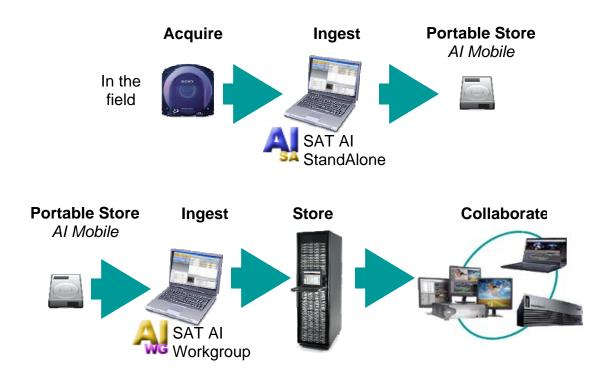
SAT AI StandAlone configuration can not transfer media to an Avid Workgroup; transfer to an Avid Unity workspace requires the SAT AI AutoIngest Workgroup configuration and SAT Transfer License dongle.
